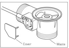
Set the position of the operating lever where the cable connects at 12 o'clock Using a tool for leverage remove the cable collar from the bath waste section and carefully release the cable from the operating lever.
