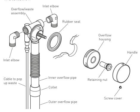
The length of the overflow pipe can be adjusted by pulling apart or pushing together the inner and outer overflow pipes.
