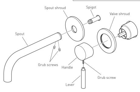
Slide the shroud over the valve, push onto the wall until it makes contact.
