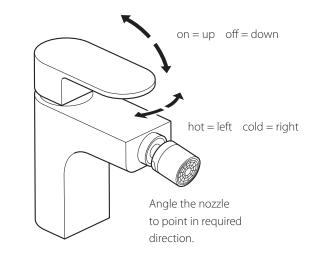
Moving the mixer lever upwards/downwards will increase/decrease the flow of water. Moving the mixer lever from right to left will increase the water temperature.
