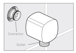
Tighten the grub screw on the underside using a hex key.
