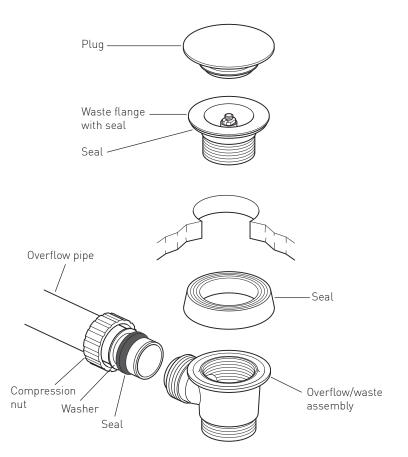
Push the seal onto the waste assembly
