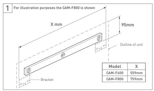
Decide on the position and height of the unit. The recommended basin height is between 800 and 900mm from floor to top of basin. Mark the bracket fixing holes onto the wall. **NOTE**: The dimensions are for the maximum width over the brackets.
