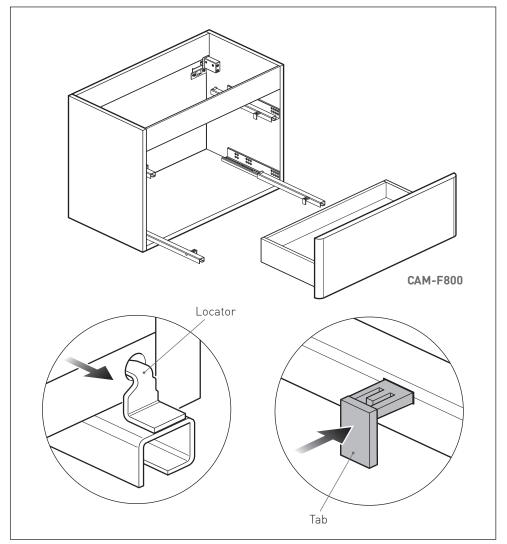
Place the drawer onto the bottom extended runners.
