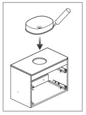
Fix basin by applying silicone on the outer edge of the basin.
