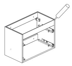
Apply silicone non-acidic to the side and front edges of the unit. Carefully position the basin down onto the unit ensuring that it is centrally positioned and flush at the back.
