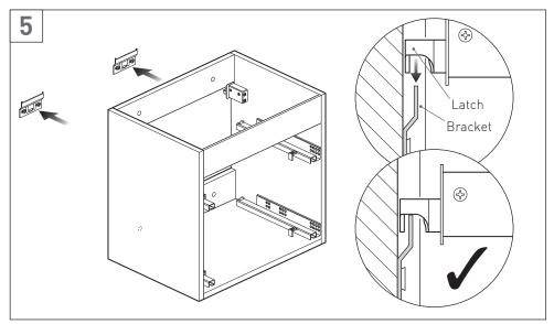
With two people lift the unit over and onto the brackets, make sure that both latches are over the brackets before releasing the unit.
