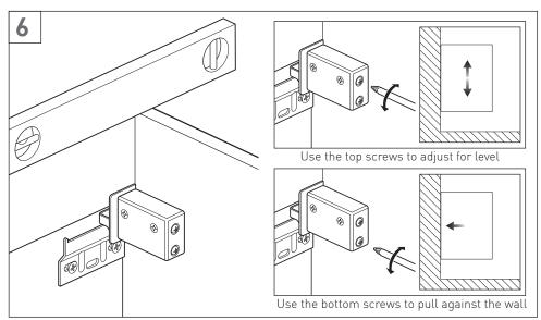
Check the unit is level. If leveling is required, use the top screw on both sides to lower or lift the unit.
