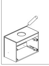
Apply a bead of silicone along the back and sides of the countertop.
