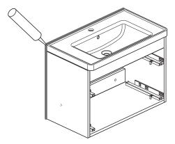
Apply a bead of silicone along the back and sides of the basin.
