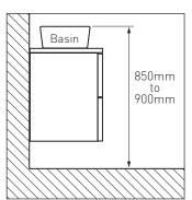
Recommended install heights We recommend installing these vanities onto solid walls. For installations onto non solid walls, consult the diagram below.
