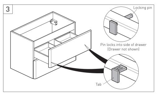
Remove the drawers prior to fitting the unit on to the wall. Pull out a drawer so it's fully extended. On the underside of the runners, push each tab towards the centre of the unit until you hear a click.
