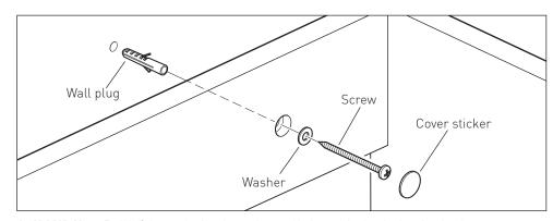
**Solid Walls -** Drill  $\emptyset$  8mm holes into the wall through the holes in the braces, insert a wall plug, washer and screw through each hole. Place the adhesive sticker over the hole.
