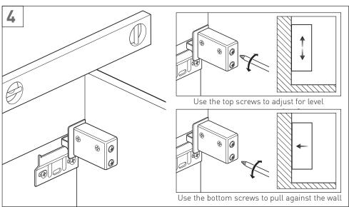
Check the unit is level. If leveling is required, use the top screw on both sides to lower or lift the unit.
