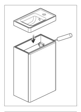
Apply a bead of silicone along the back and sides of the basin.
