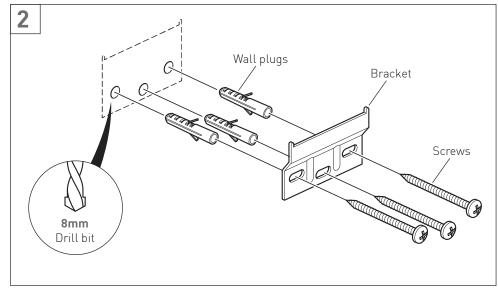
Drill  $\emptyset$  8mm holes, insert the wall plugs and screw on the brackets.
