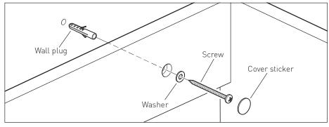
Solid Walls - Drill  $\emptyset$  8mm holes into the wall through the holes in the bottom brace, insert a wall plug, washer and screw through each hole. Place the adhesive sticker over the hole.
