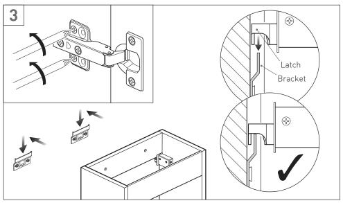
Remove the door of the vanity by unscrewing the hinges. With two people lift he unit over and onto the brackets, make sure that the that both latches are over the brackets before releasing the unit.
