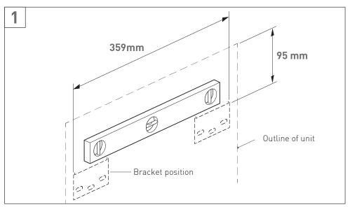
Decide on the position and height of the unit. The recommended basin height is between 800 and 850mm from floor to top of basin. Mark the bracket fixing holes onto the wall. **NOTE:** The dimensions are for the maximum width over the brackets.
