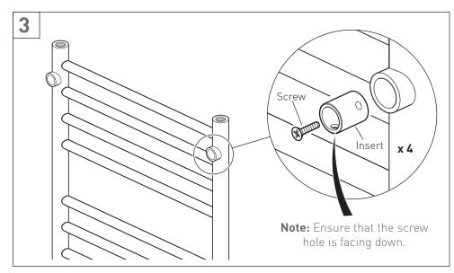
Using the counter sunk screw fix the bracket insert onto each keyhole on the heated towel rail, ensuring the screw hole is facing down.
