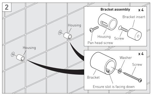
Disassemble the wall brackets and attach each housing to the wall using a washer and screw. Ensure the slot is facing down on each bracket housing.
