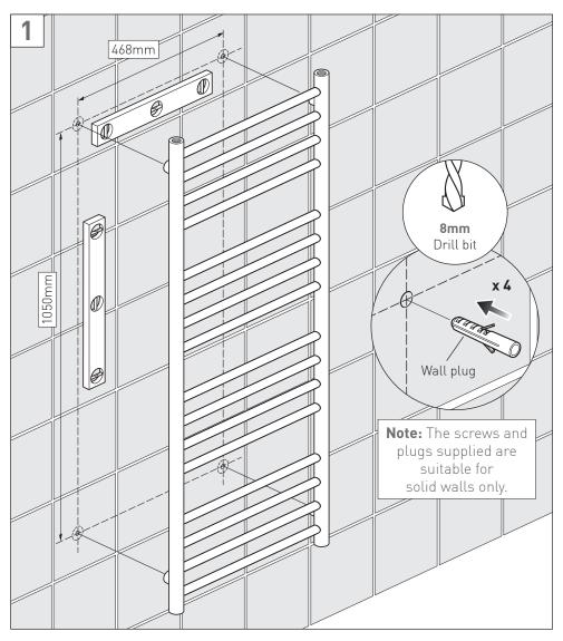
Measure and note the distance between the centres of the four mounting keyholes. Determine the desired location of the heated towel rail.
