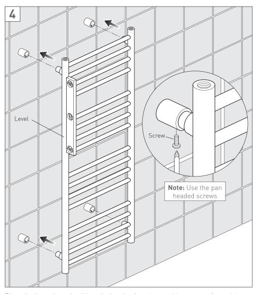
Place the heated towel rail into the bracket housings and insert one of remaining screws into each bracket lining up both holes. Use a level to make sure that the rail is vertical, the brackets have 10mm of adjustment.
