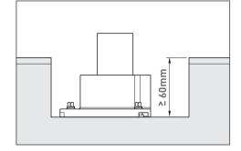
There are 3 fixing positions and 3 levelling halts
