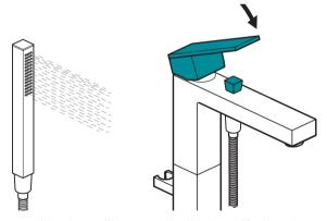
Handset will automatically shut off when the flow handle is turned off.
