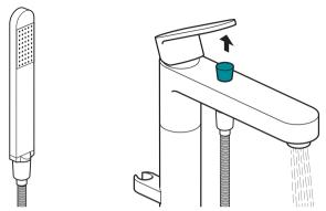
Pull up the diverter handle to change flow to handset.
