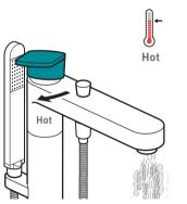
Moving the mixer lever to the left will increase the water temperature.
