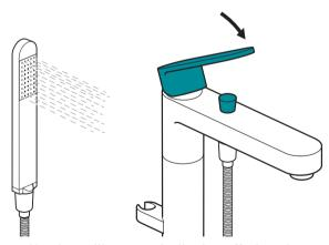
Handset will automatically shut off when the flow handle is turned off.
