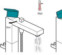
Moving the mixer lever to the left will increase the water temperature.
