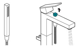
Pull up the diverter handle to change flow to handset.
