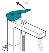
Moving the mixer lever upwards/downwards will increase/ decrease the flow of water.
