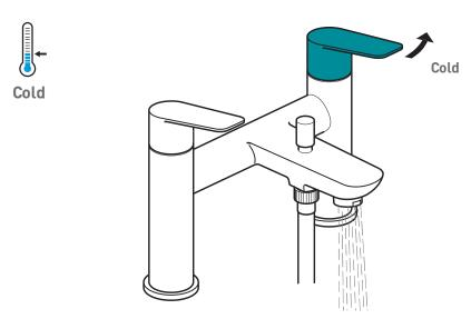
Turning the cold handle to the right will increase the flow of cold water.
