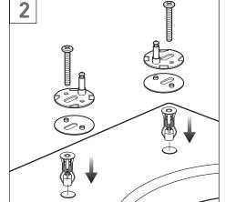
Fit the plugs into the holes on the WC pan. Place each scew through the bracket, washer and screw into the plug.
