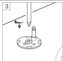
Tighten the screws. **NOTE.** Don't fully tighten at this stage as adjustment is required.
