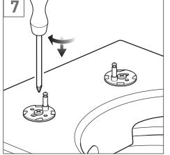
Tighten the screws in a clockwise direction (Do not overtighten).
