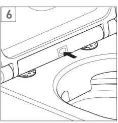
Take off the toilet seat by lifting the seat while holding the release button.
