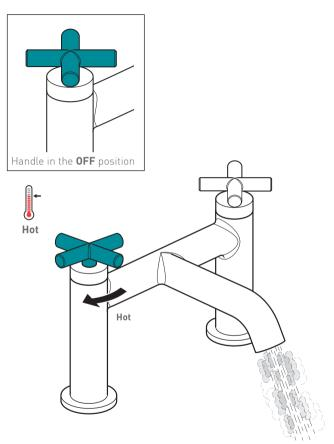
Turning the hot handle to the left will increase the flow of hot water.
