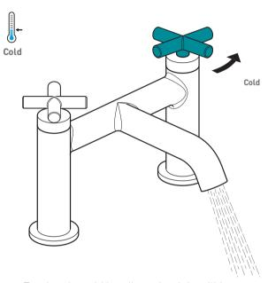
Turning the cold handle to the right will increase the flow of cold water.
