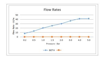
The flow rate displayed is calculated using ideal system conditions. This result should only be taken as an indication as the flow rate may vary depending on the specific in-situ configuration.
