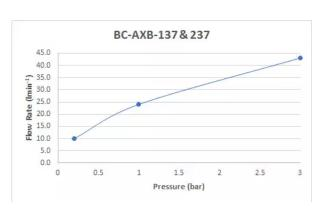
The flow rate displayed is calculated using ideal system conditions. This result should only be taken as an indication as the flow rate may vary depending on the specific in-situ configuration.
