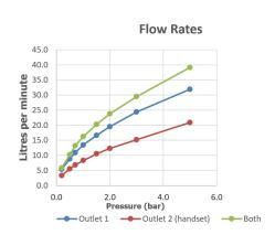
The flow rate displayed is calculated using ideal system conditions. This result should only be taken as an indication as the flow rate may vary depending on the specific in-situ configuration.
