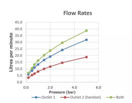
The flow rate displayed is calculated using ideal system conditions. This result should only be taken as an indication as the flow rate may vary depending on the specific in-situ configuration.
