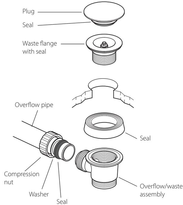
Push the seal onto the waste assembly
